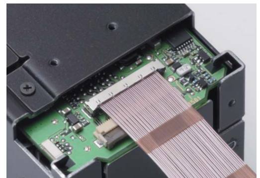
Micro coaxial cable can be used for digital interface.
